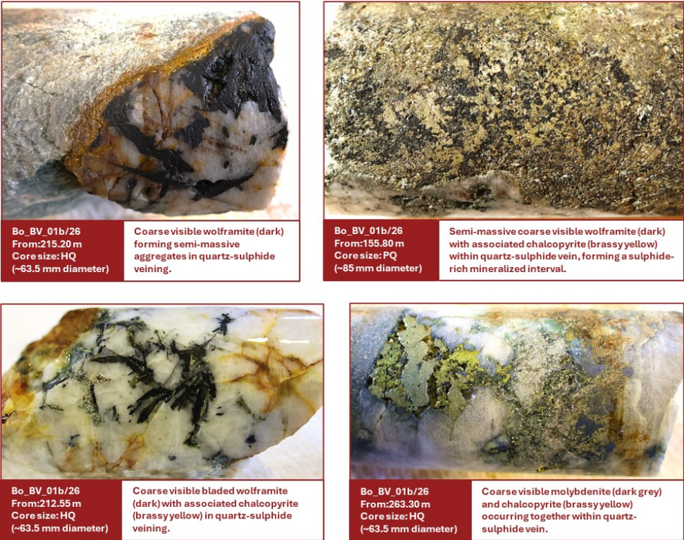
Figure 2 (above): Representative drill core from hole Bo_BV_01b
