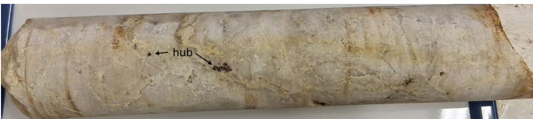
AT25-01 96.8 ft. Hubnerite masses in coarse milky quartz. Core diameter is 2 inches.
