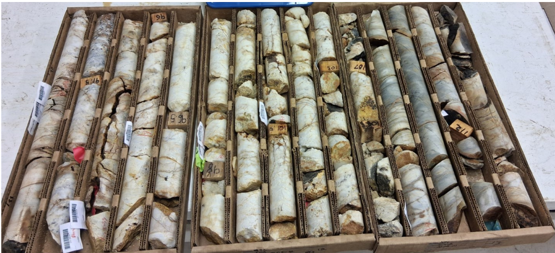
AT25-01 88 ft to 115 ft showing No.5 quartz-hubnerite-tetrahedrite-pyrite-calcopyrite vein intercept.
