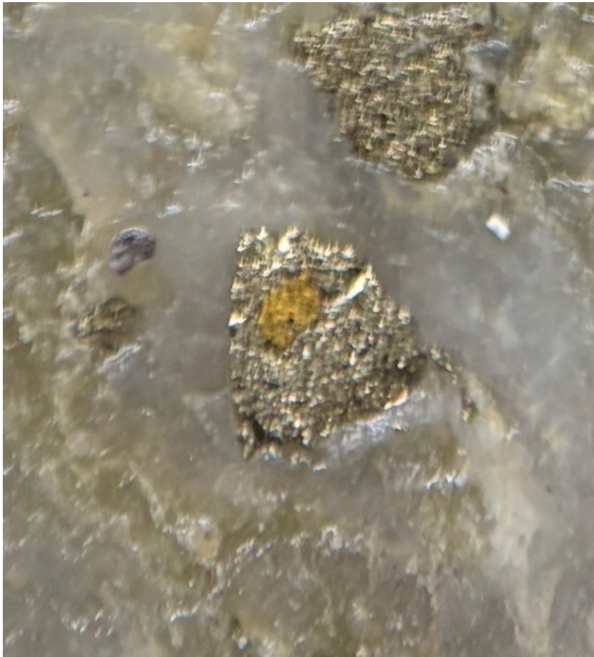
Photo 3: Gold Contained in Pyrite Drill Hole BHC-26-13 at 165.85 m.
