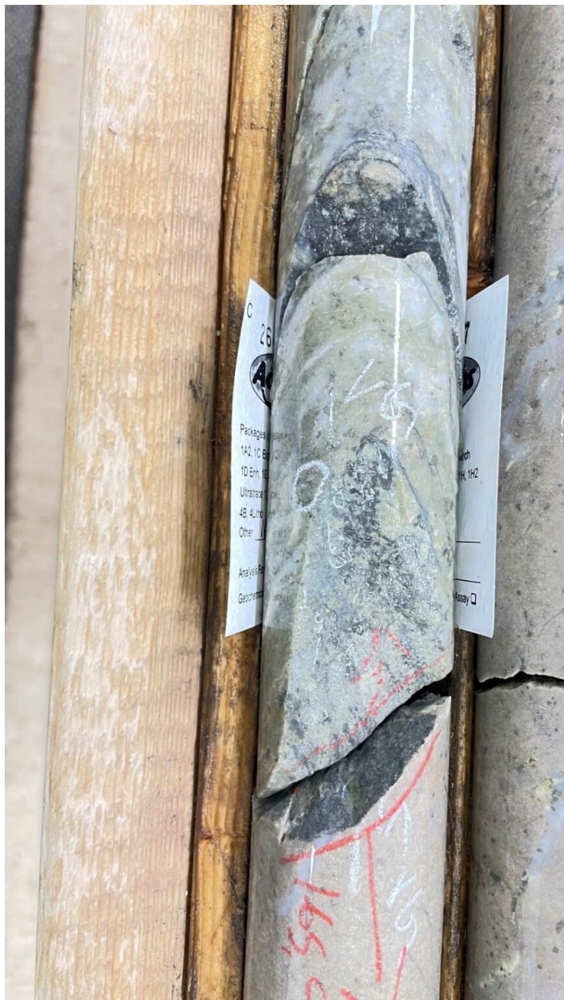
Photo 1: Gold Identified in Drill Hole BHC-13 at a Depth of 165.85 Meters. Note labeled V6
