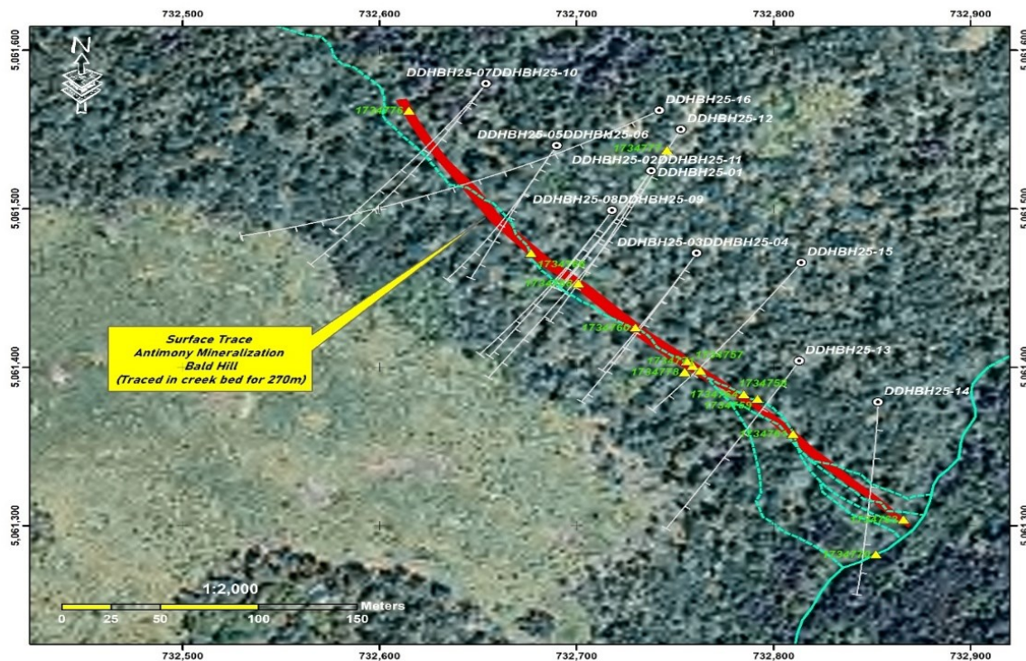
Figure 1: Drillhole Locations on the Bald Hill Antimony Main Zone. Note the location of drill holes and surface exposures along the trend of the mineralized zone indicated by triangles.
