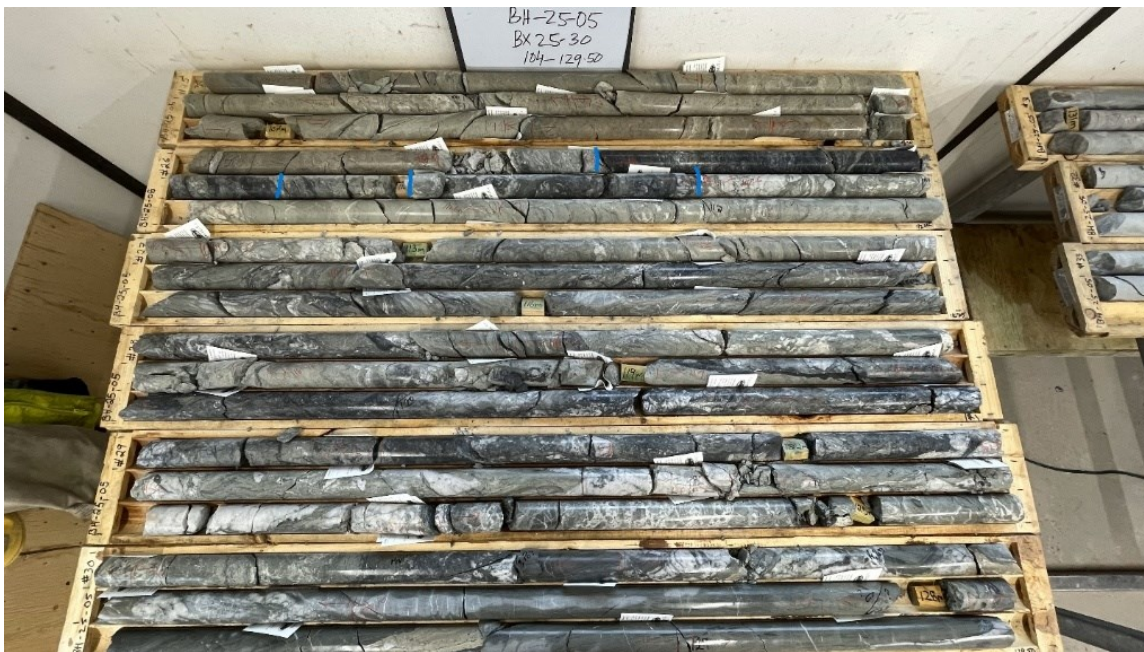
Photo 1: Mineralized Section in Drill Hole BH-25-05. Note stibnite is identified over 20 meters in this hole.
