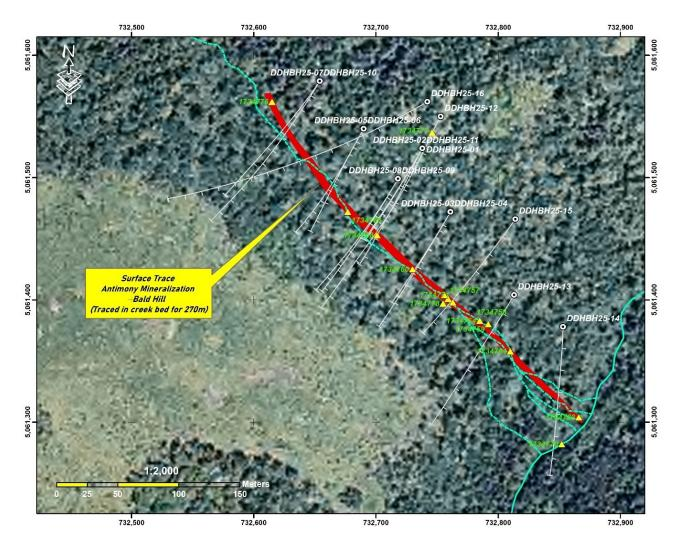
Figure 1: Drillhole Locations on the Bald Hill Antimony Main Zone. Yellow triangles represent locations of massive stibnite occurrences on surface. The surface trace of the mineralization is shown in red while drill hole locations are shown by circles. Note: only the drill holes in Antimony Resources recently completed Phase One Program are shown for clarity.
