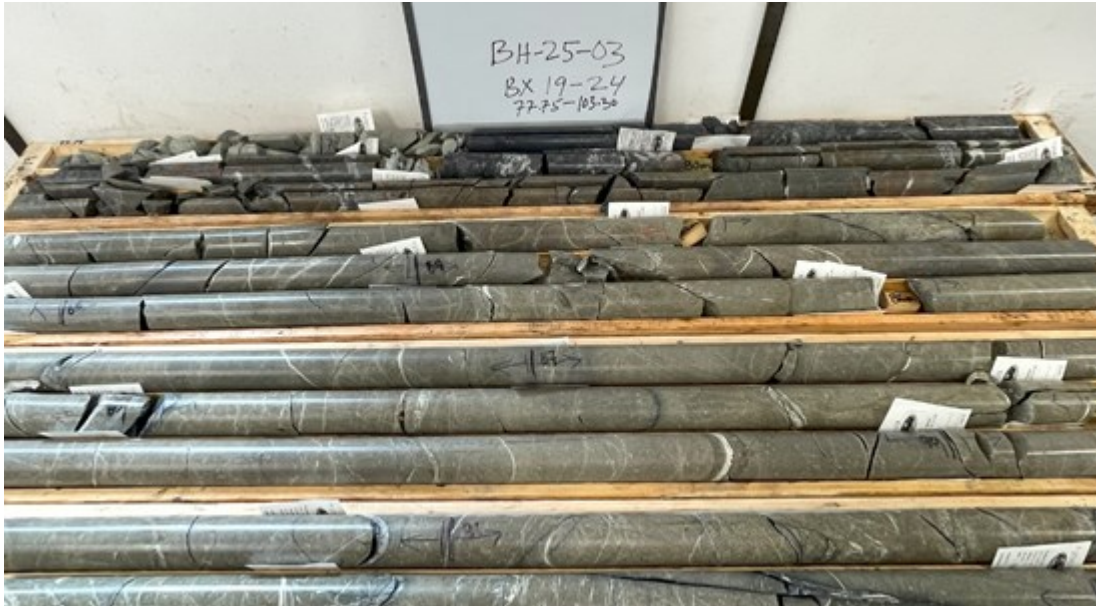
Photo 1: Drill Hole BH-25-03. Massive Antimony Bearing Stibnite Mineralization in Siltstone. Note: Dark sections Contain Antimony Mineralization.
