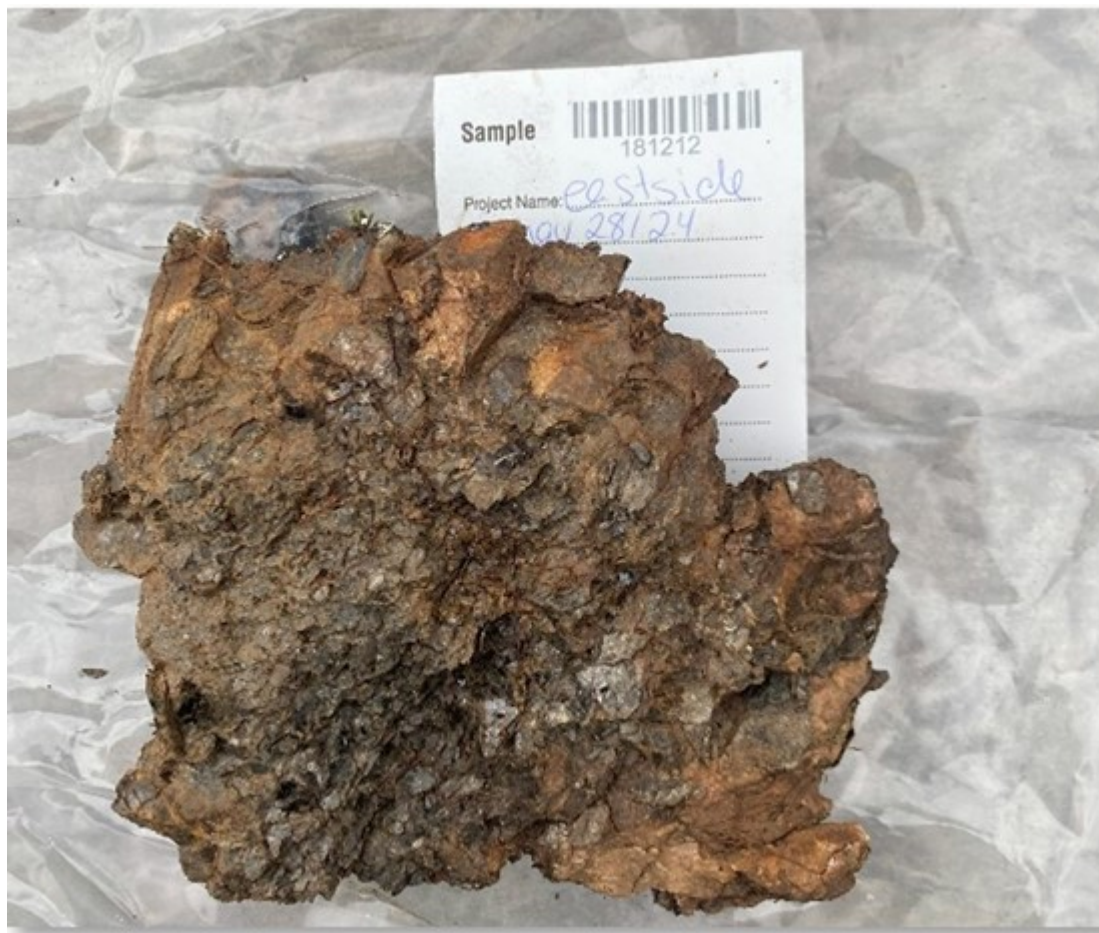
Figure 4 – Uranium sample 181212 displaying 0.06 wt% U3O8 hosted within biotite-rich pegmatite
