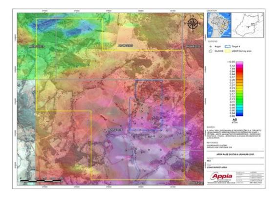
Figure #1 – The figure showcases a Lidar survey area displayed over satellite imagery, with the Analytical Signal superimposed. The blue polygon highlights the Target #4 area, while the white dots represent the locations where auger drilling has been carried out by the vendors.
