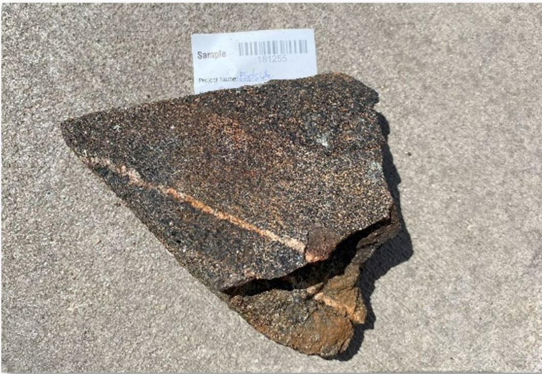
Figure 3 – Uranium sample 181255 displaying 0.07 wt% U 3 O 8 hosted within granodiorite
