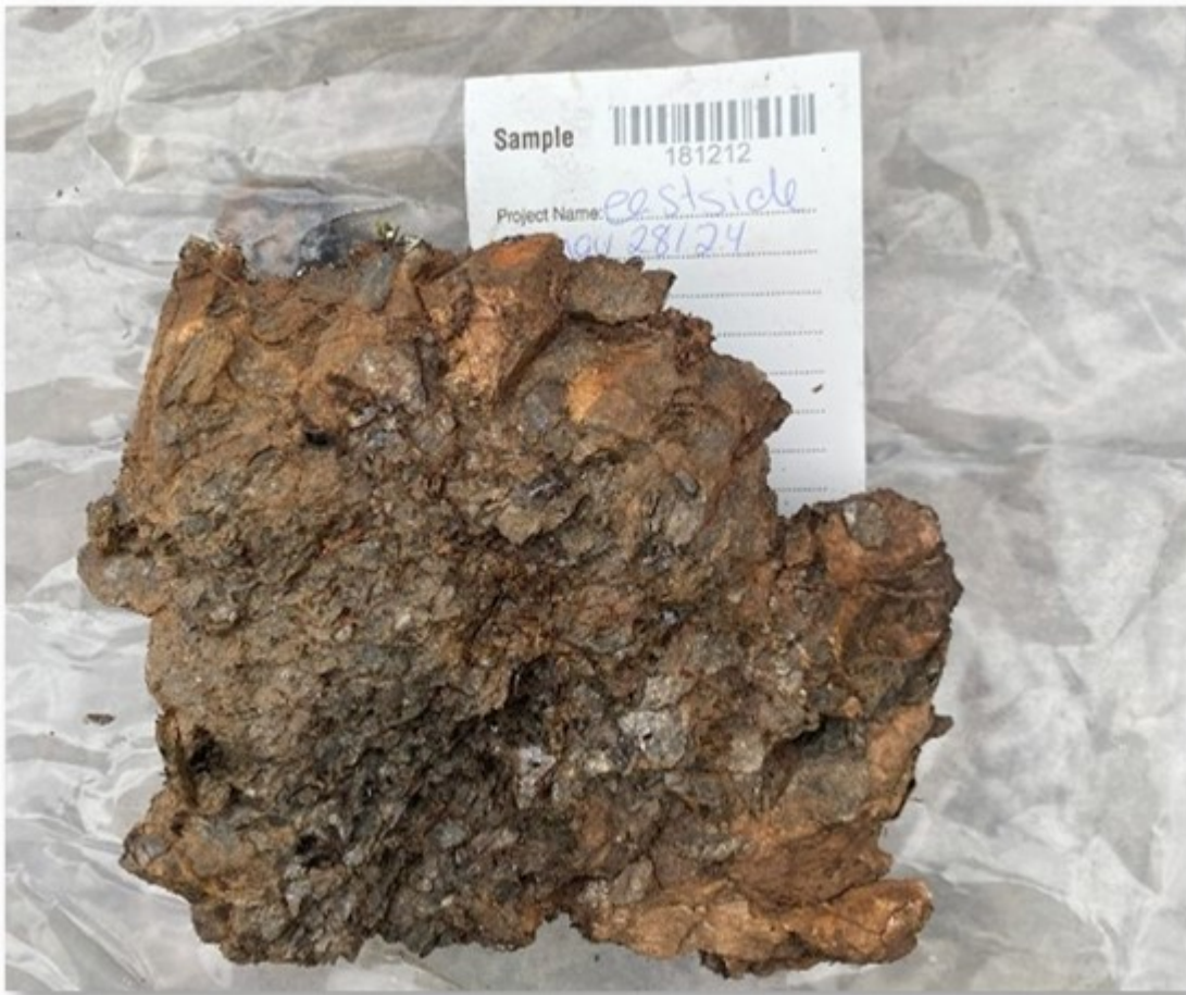
Figure 4 – Uranium sample 181212 displaying 0.06 wt% U 3 O 8 hosted within biotite-rich pegmatite
