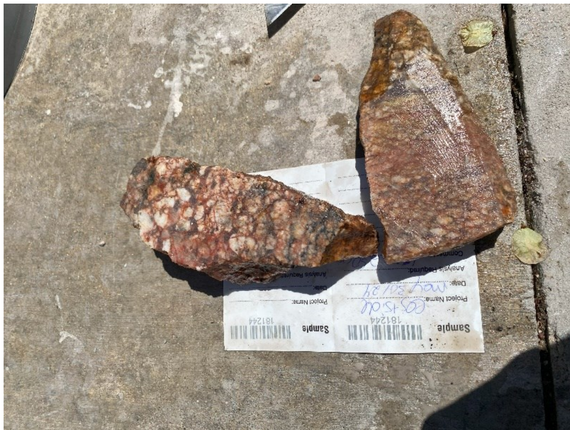
Figure 5 – Rare earth element sample 181244 displaying 0.14 wt% TREO hosted within granite
