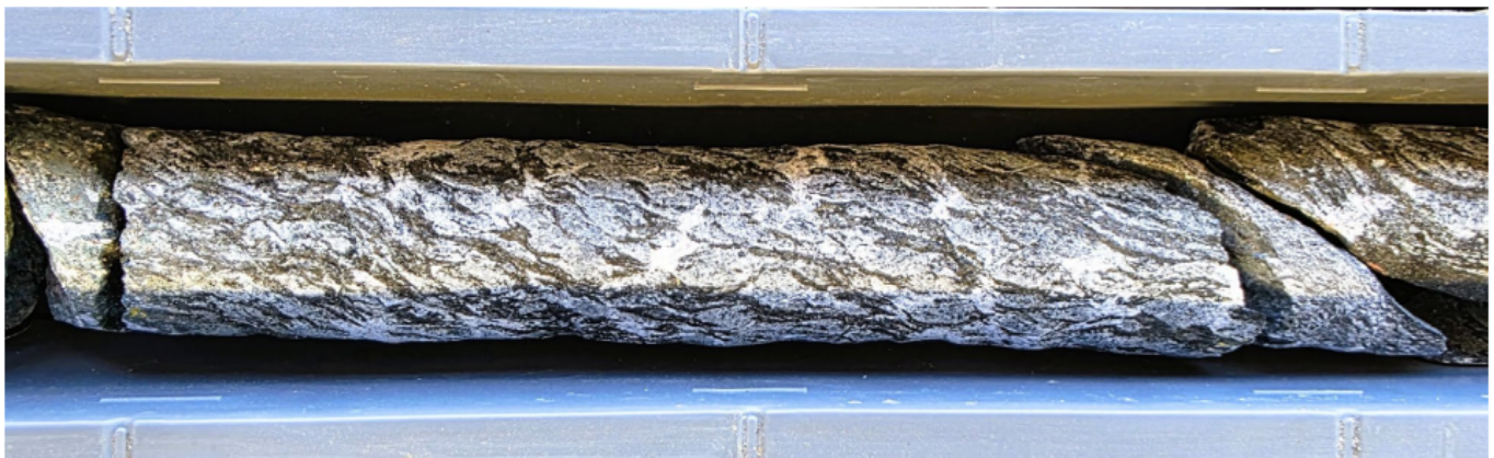
Figure 4: OV176 core (centred on 146.4m) showing strong foliation, brecciation, and metasomatic alteration.
