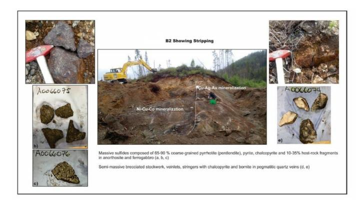
Massive sulfides composed of 65-90 % coarse-grained pyrrhotite (pentlendite), pyrite, chalcopyrite and 10-35% host-rock fragments in anorthosite and ferrogabbro (a, b, c)
