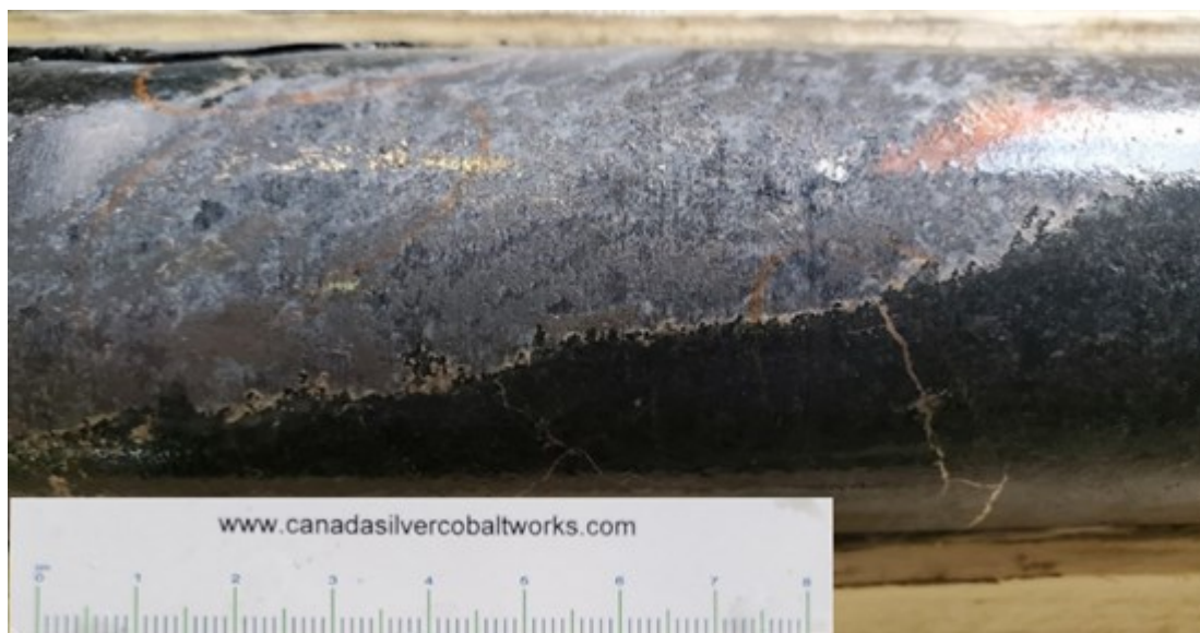
Figure 1: Close-up of mineralization in hole CS-21-61 (30,416.91 g/tonne Ag). One can see the intense Cobalt mineralization occurring as the dark grey minerals within the vein. The bright silver is located within the cobalt clusters as well as lining the edge of the vein and radiating outwards.
