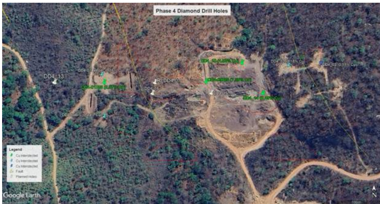
Figure 5: Phase 4 Diamond Drill Hole Positions with Copper Intersections Weight Percentage and planned drill holes at the white pins.
