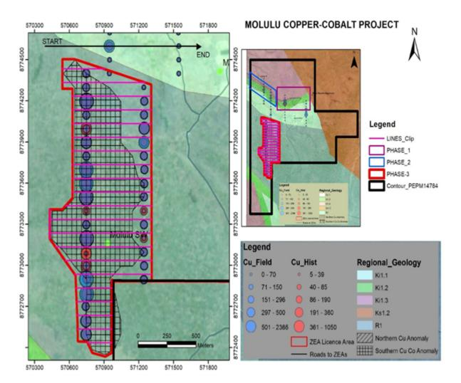
During the mapping and geophysics surveys, two new copper anomalies were discovered directly south of the Phase 1 area. These new areas, known as Phase 1a and Phase 1b, will be included in the current IP programme. The Company believes that this will further increase the tonnage to the already known copper resource base.
