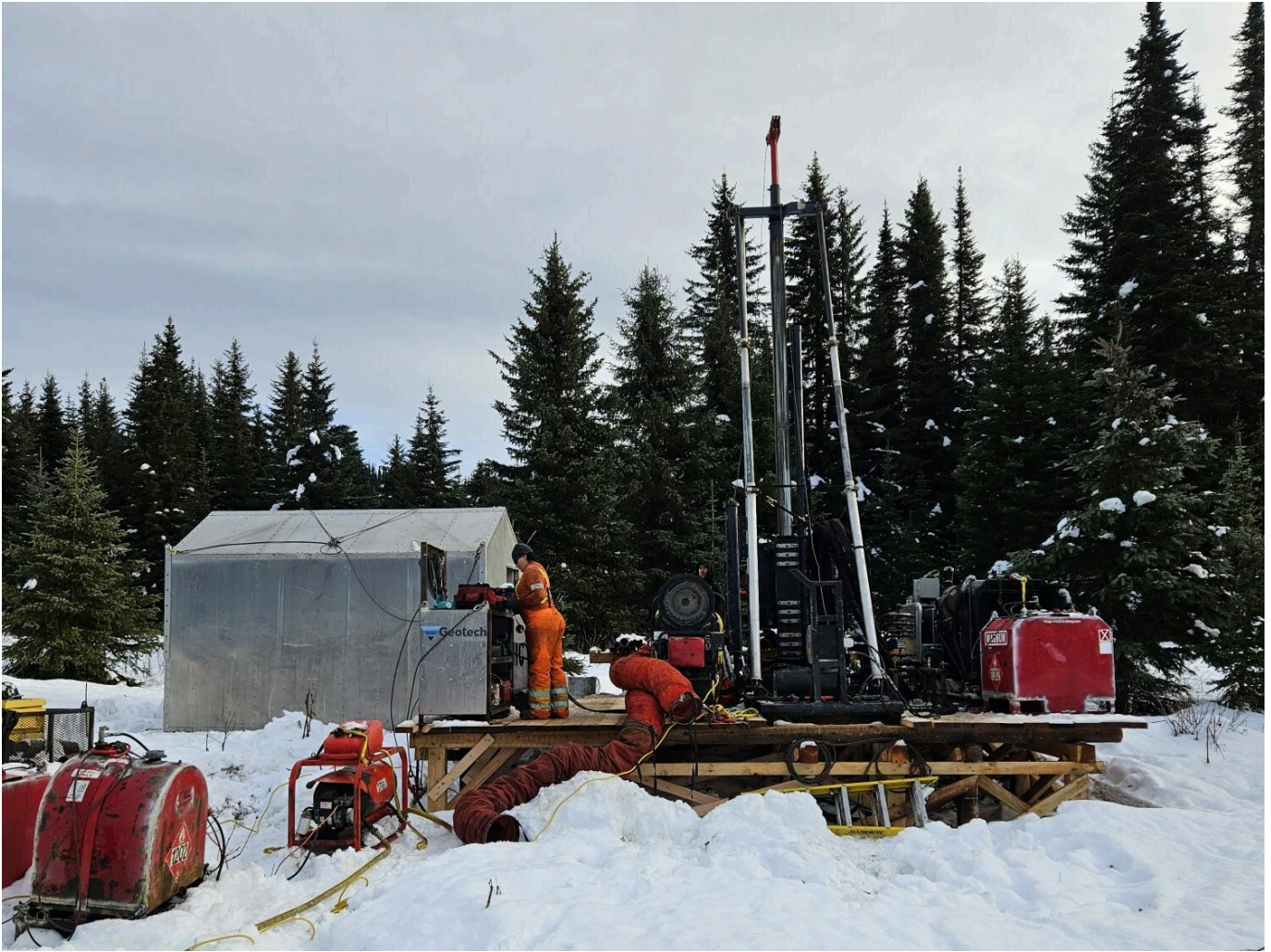
Image 1: Heli-Sonic Overburden Drilling in PFS Tailings Option Study Area (CNW Group/Defense Metals Corp.)
