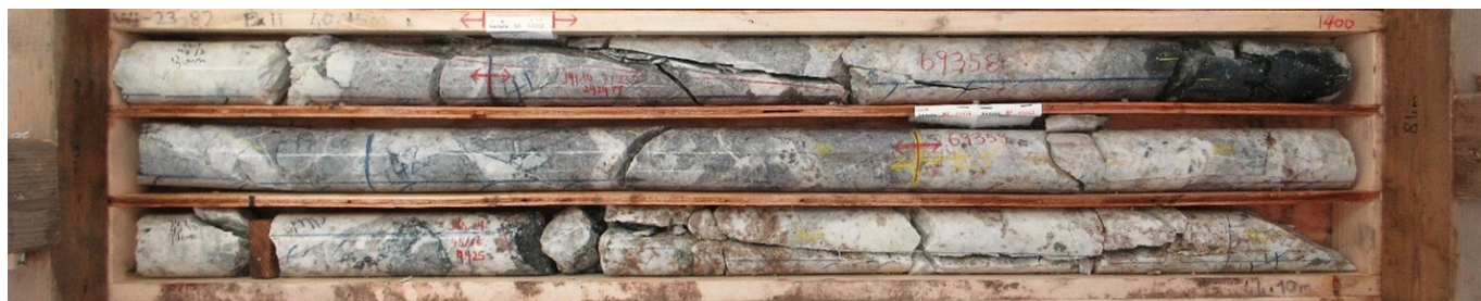
Image 2: REE Mineralized-Xenolithic Dolomite West Pit Wall Radiometric Anomaly (WI23-82, 40.75-44.10 m) (CNW Group/Defense Metals Corp.)
