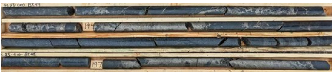
Photo – 1: Drillhole GL23010 Disseminated, Semi-Massive Sulphide Textures at drillhole depth ~193-198 meters
