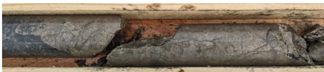
Photo - 4: Drillhole GL23008 Massive Sulphide Vein with
