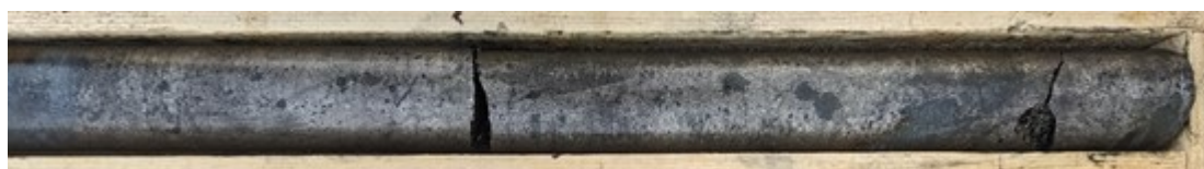
Photo - 3: Drillhole GL23009 Semi-Massive Sulphide with Host Rock Inclusions at drillhole depth ~379 meters
