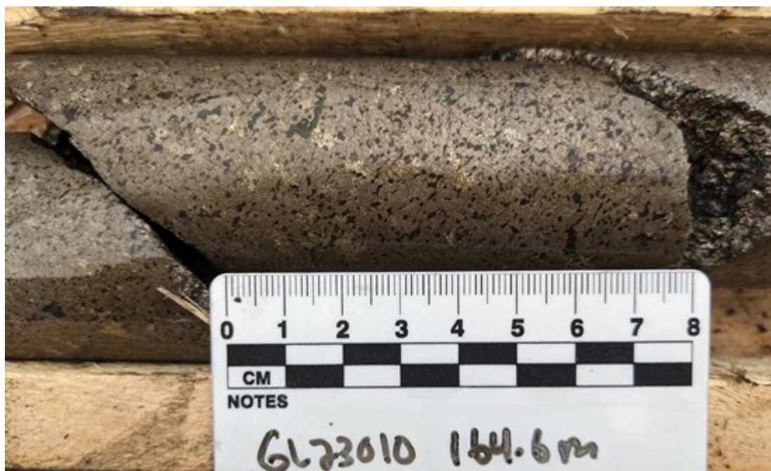
Photo - 2: Drillhole GL23010 Disseminated Coarse Pentlandite in Semi-Massive Sulphide Host at drillhole depth 164.6 meters
