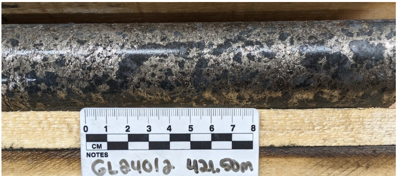
Photo – 1: Detailed Photo Interstitial – net-textured sulphide mineralization; drillhole GL24012 @ 421.50 meters
