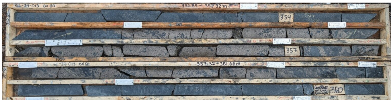
Photo – 2: Semi-Massive to Massive Sulphide Mineralization (cut core); drillhole GL24013 @ ~354.50 – 358.50 meters
