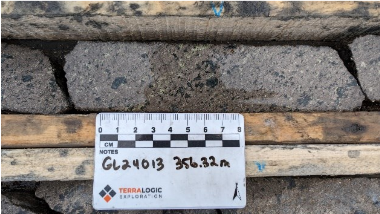
Figure 3a – Coarse granular pentlandite @ 356.32m; 2.65% Ni, 0.62% Cu, 0.21% Co
