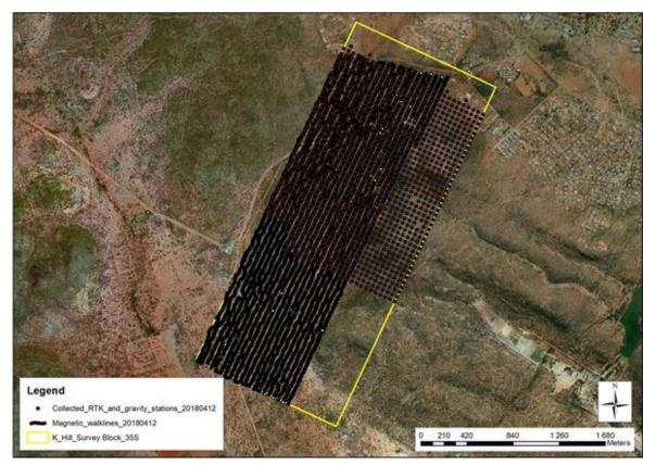
Completed RTK/Gravity stations, and Magnetic Walk-lines as of April 12, 2018.
