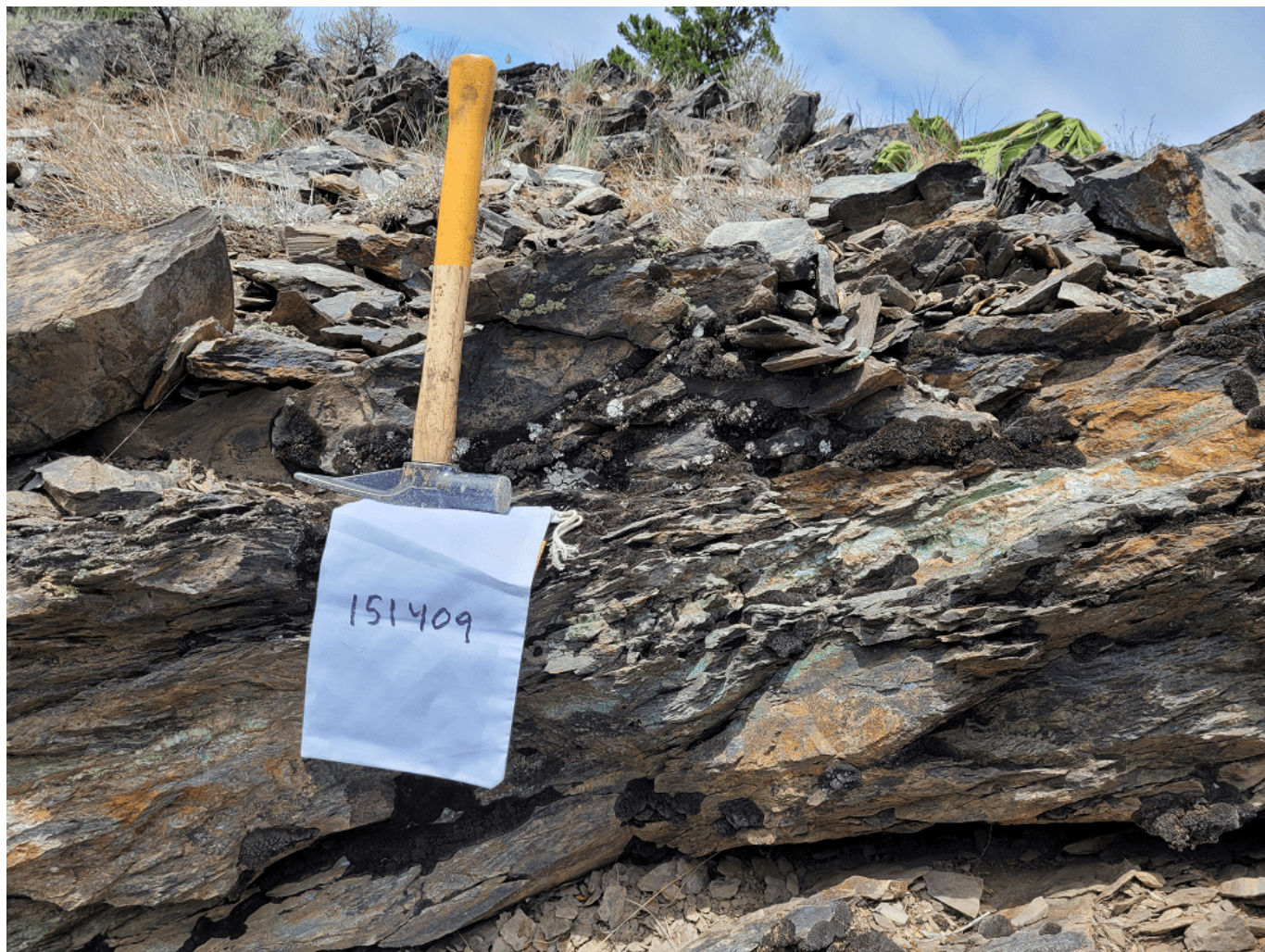
Figure 3. Sample 151409: 3.59 % Cu, 112 g/t Ag, 1.63 g/t Au. Rock sample from outcrop within historical mineralized trench located along strike between the central and southern showings.
