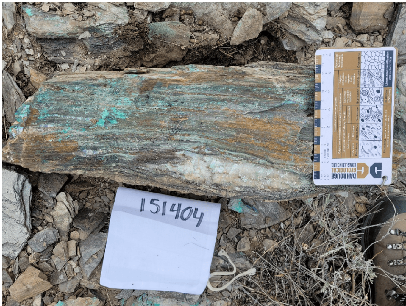
Figure 2. Sample 151404: 0.61 % Cu, 48.2 g/t Ag, 2.44 g/t Au. Rock sample with copper oxide staining located in a newly discovered historical pit in the south of the property.
