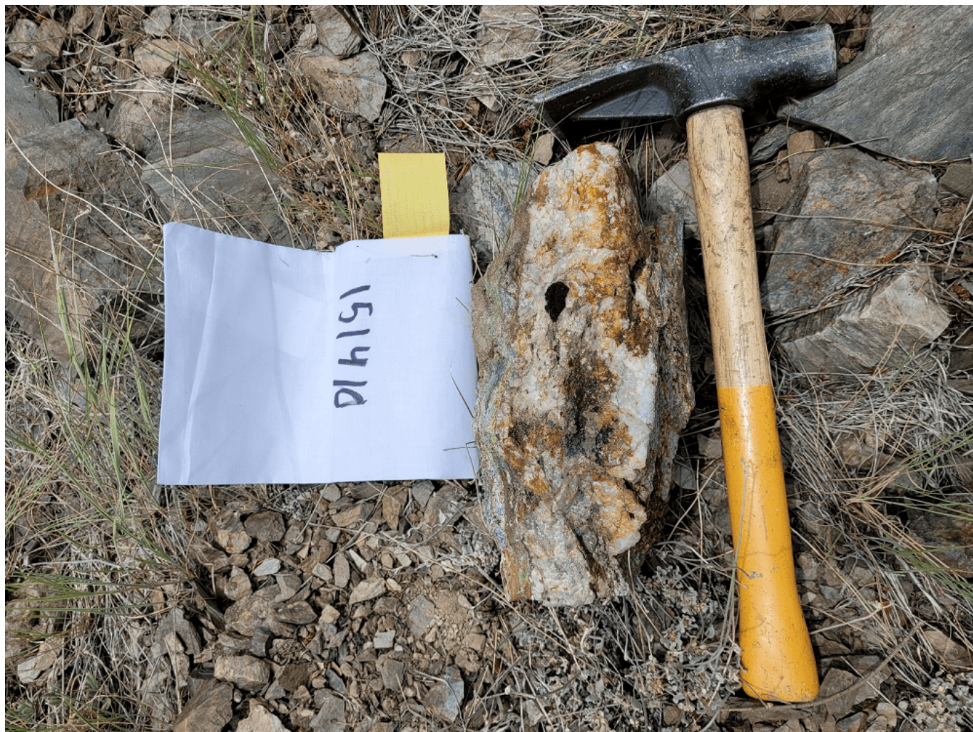
Figure 4. Sample 151410: 4.93 % Cu, 87.8 g/t Ag, 17.6 g/t Au. Rock sample from historical mineralized trench located along strike between the Jackson/Baker Adit and Anderson Occurrence.
