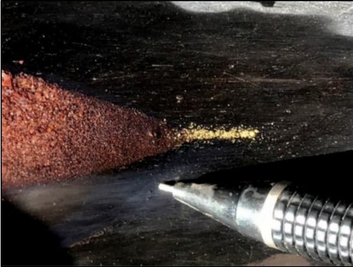
Figure 1 Visible Gold from Panning of Epithermal Quartz Vein Channel Sample – Nava Zone (1) mineralization in the photograph is not necessarily representative of the mineralization hosted on the property (CNW Group/Goldplay Exploration Ltd)
