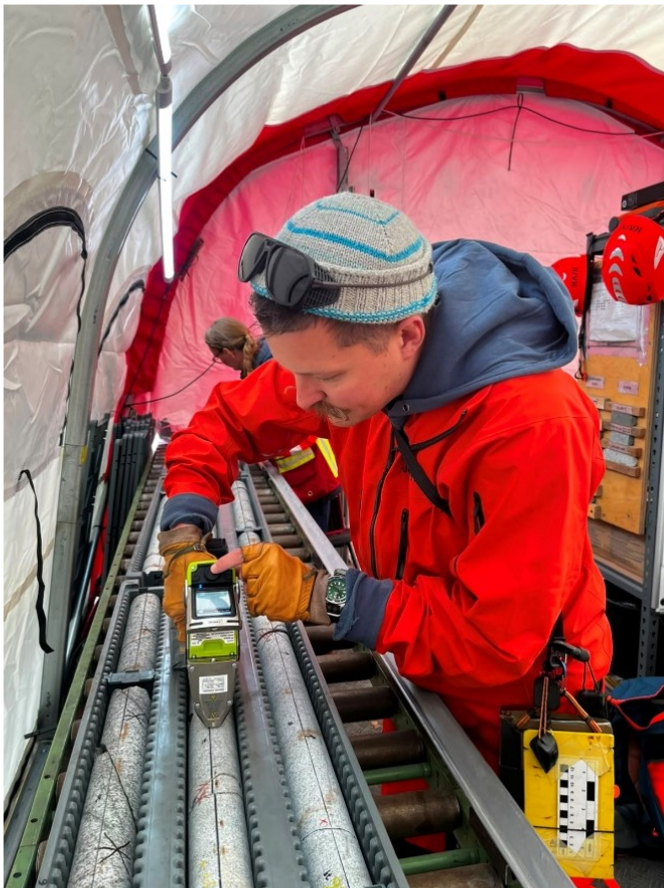
XRF Measurements Conducted – Greenland Mines Ltd. geologist
