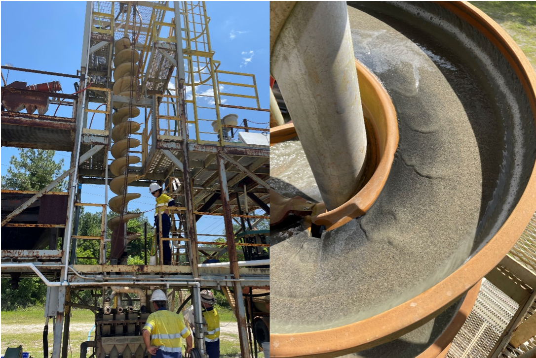
Figure 2 – MG 12 Spiral from Mineral Technologies and Halleck Creek Feed in the Spiral
