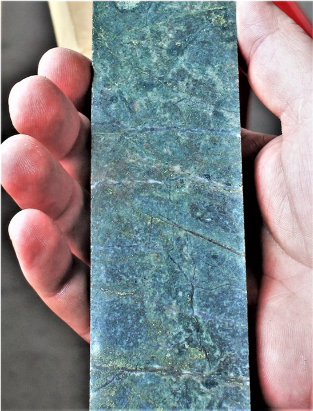
Figure 5: Example of core from 2021 Drilling at Dillard: MPD-21-035: Altered-brecciated andesite with disseminated and fine veinlets of chalcopryrite-pyrite associated
