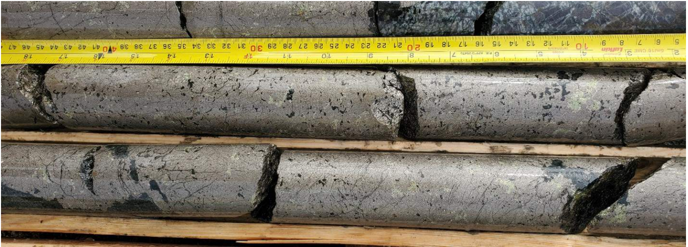
Figure 1: Massive sulphide mineralization in BDF22-003 at 36.69 m to 41.00 m.
