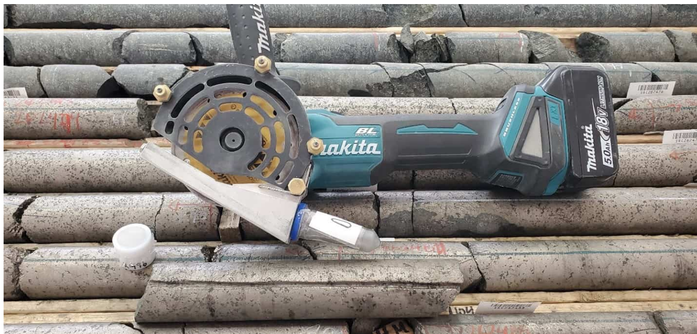
Figure 6: Direct rock sampler, sampled core and example sample puck from BDF22-001.
