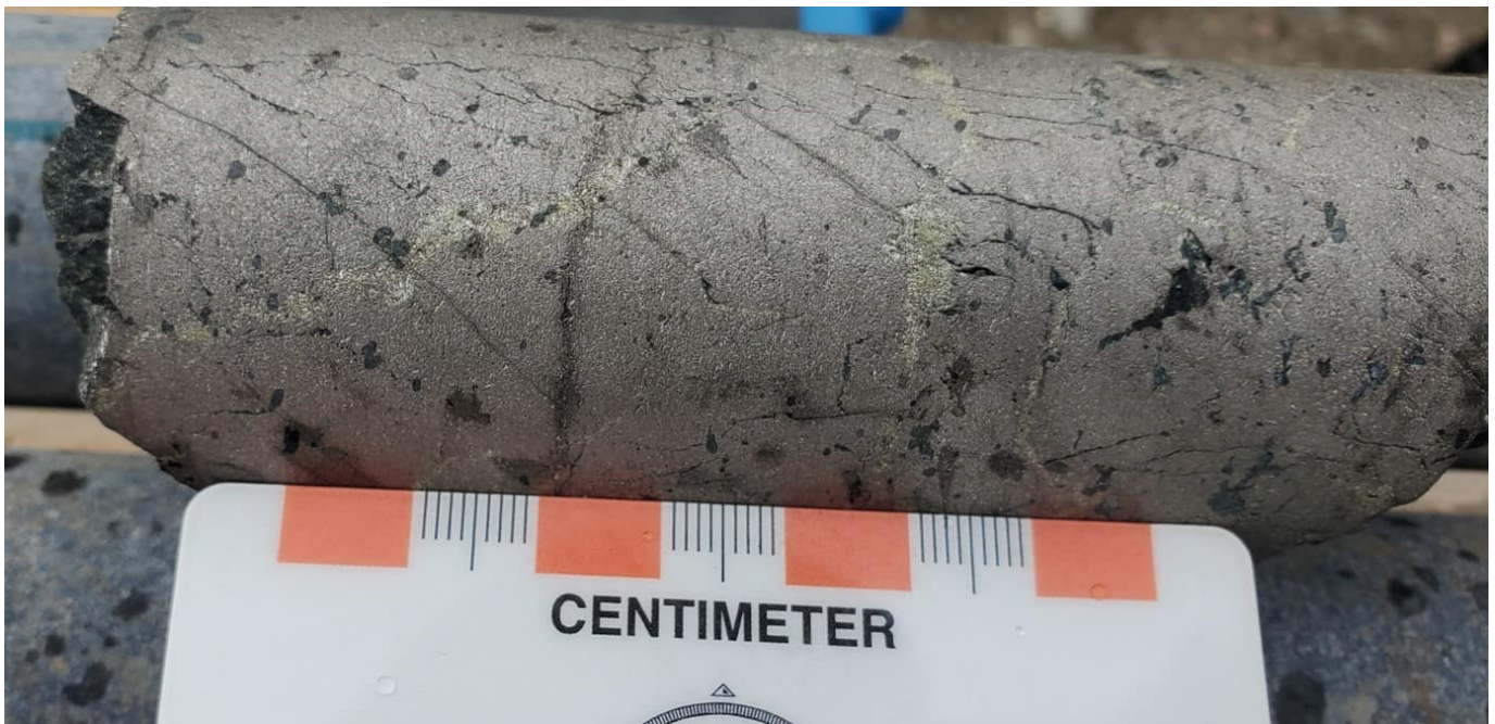
Figure 2: Close-up of loop pentlandite (light brassy mineral) within massive sulphide mineralization in BDF22-003.
