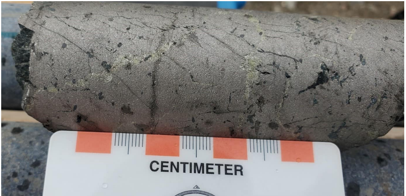
Figure 2: Close-up of loop pentlandite (light brassy mineral) within massive sulphide mineralization in BDF22-003.
