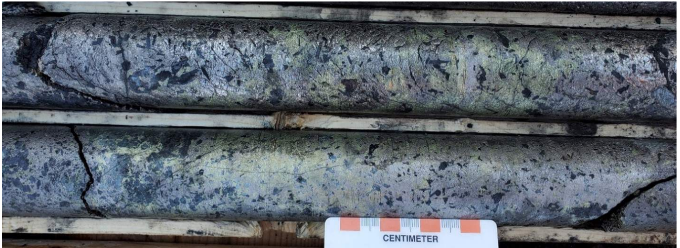
Figure 4: Zoom in on Massive Sulphide in BDF22-002 displaying observable pentlandite (nickel sulphide) and chalcopyrite (copper sulphide) with pyrrhotite (iron sulphide) mineralization.
