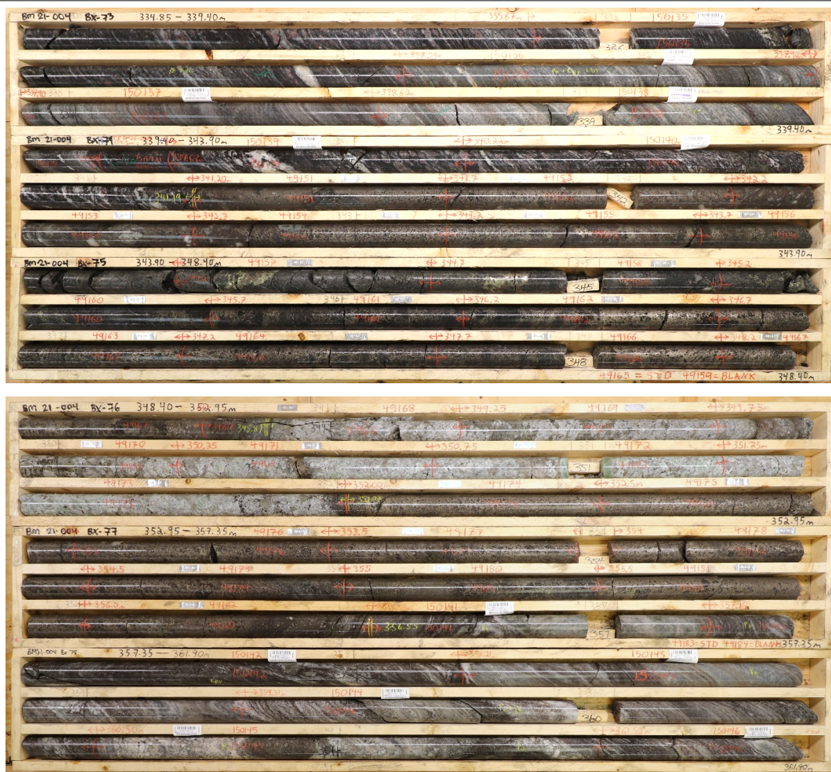
Figure 1: Drill core displaying zinc, copper, lead, silver mineralization observed in BM21-004
