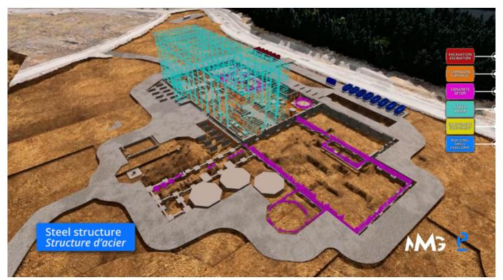
4D model of the Matawinie Mine construction timeline produced by Pomerleau using the Building Information Modeling platform, available for viewing at <a href="https://youtu.be/rNvgCVHRzEw">https://youtu.be/rNvgCVHRzEw</a>.
