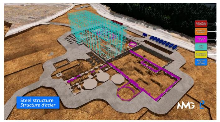
4D model of the Matawinie Mine construction timeline produced by Pomerleau using the BIM platform, available for viewing at <u>https://youtu.be/rNvgCVHRzEw</u>.
