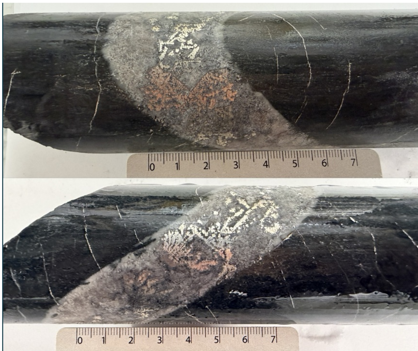
Figure 1. Core from CS-26-140W1 at approximately 404.80 metres downhole, showing native silver with plumose texture, cobalt mineralization and native-silver stringers proximal to the vein.
