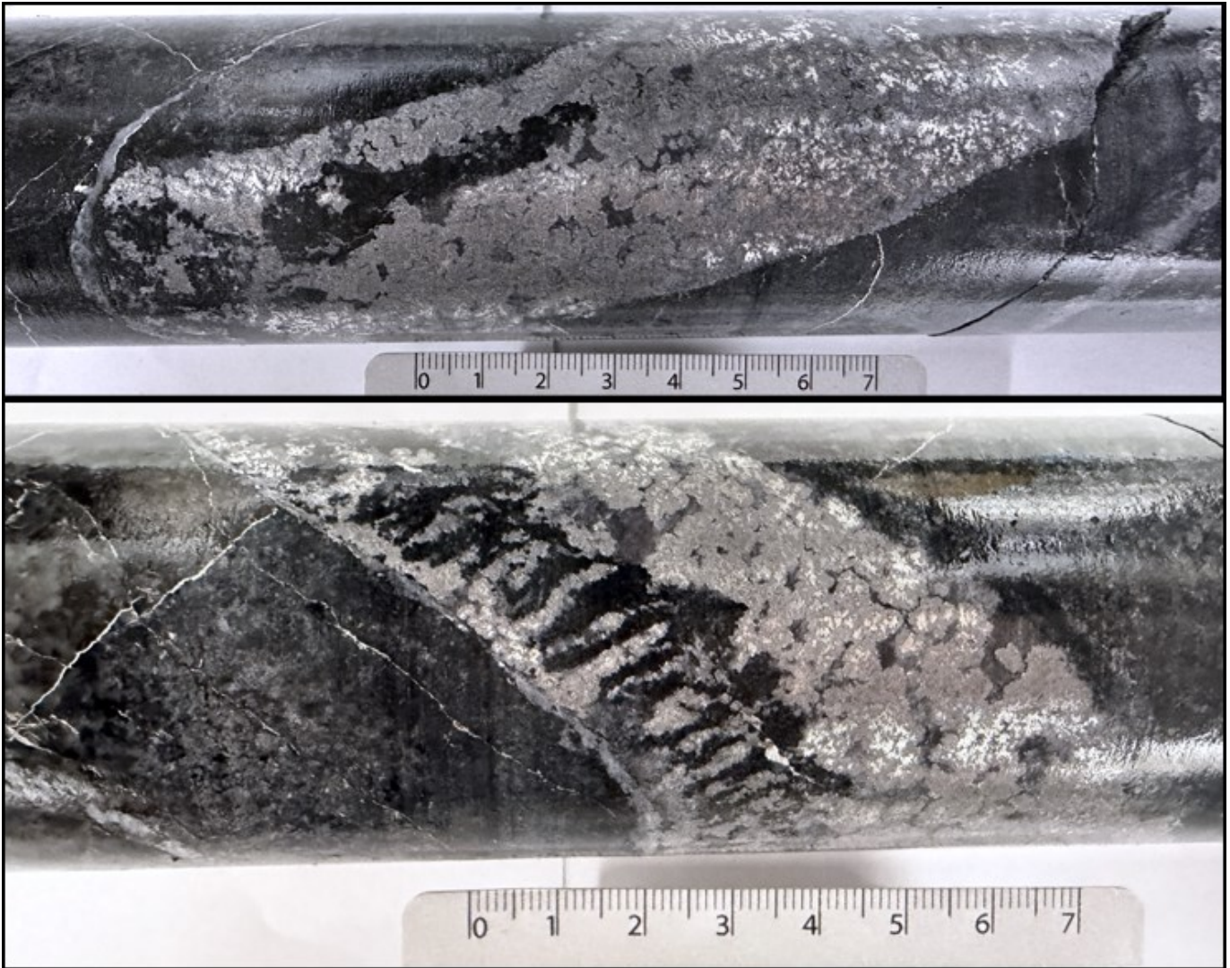
Figure 2: Close-up pictures of native silver and cobalt arsenide mineralization vein and native silver-filled fractures adjacent to vein in hole CS-21-73W3 at 480.8 metres downhole; 5 cm true width. Photo 1 – Calcite vein hosting native silver with cobalt arsenide mineralization at 480.8 metres downhole in CS-21-73W3
