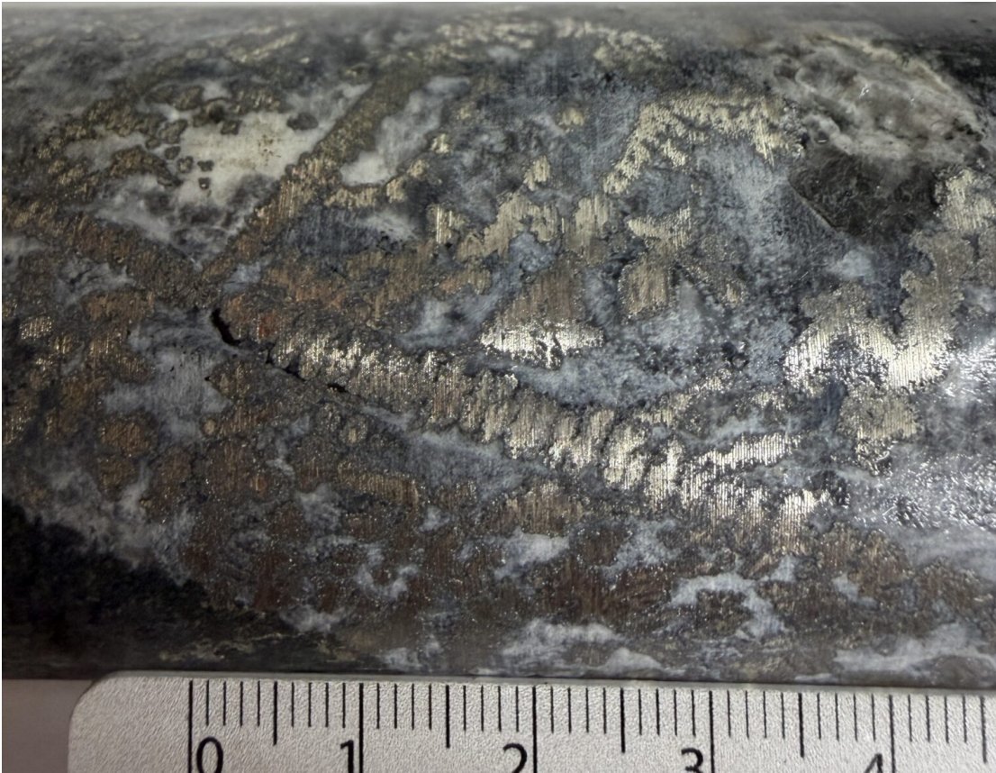
Photo 2 – Close-up of visually high-grade native silver and cobalt mineralization in hole CS-21-73W1 at 501.90 metres downhole
