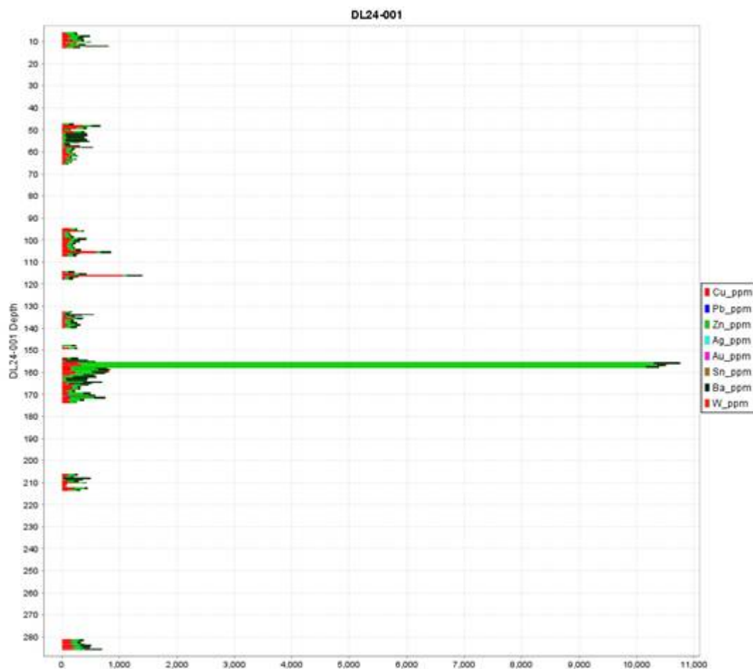
Figure 3: Diamond Drill Hole DL24-001 Multielement Correlations (A & B) Supports VMS Style Mineralisation Source. Note: For illustration purposes zinc concentration is capped at 10,000 ppm in figure 2 B; actual zinc concentrations exceed 38,000 ppm Zn.
