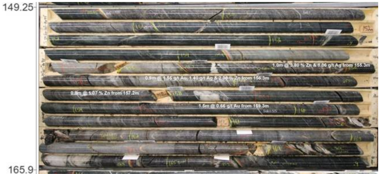
Figure 2: Photography of DL24-001 Drill Core over the interval from 155.3m to 160.8m downhole depth which returned 4.5m @ 0.64g/t Au from 156.3m and 5.5m @ 1.21 % Zn from 155.3m. Photograph markup shows additional high grade intervals such as 1.0m @ 3.80 % Zn & 1.06 g/t Ag from 155.3m, 0.9m @ 1.55 g/t Au, 1.40 g/t Ag & 2.08 % Zn from 156.3m, 0.8m @ 1.07 % Zn from 157.2m and 1.5m @ 0.66 g/t Au from 159.3m.
