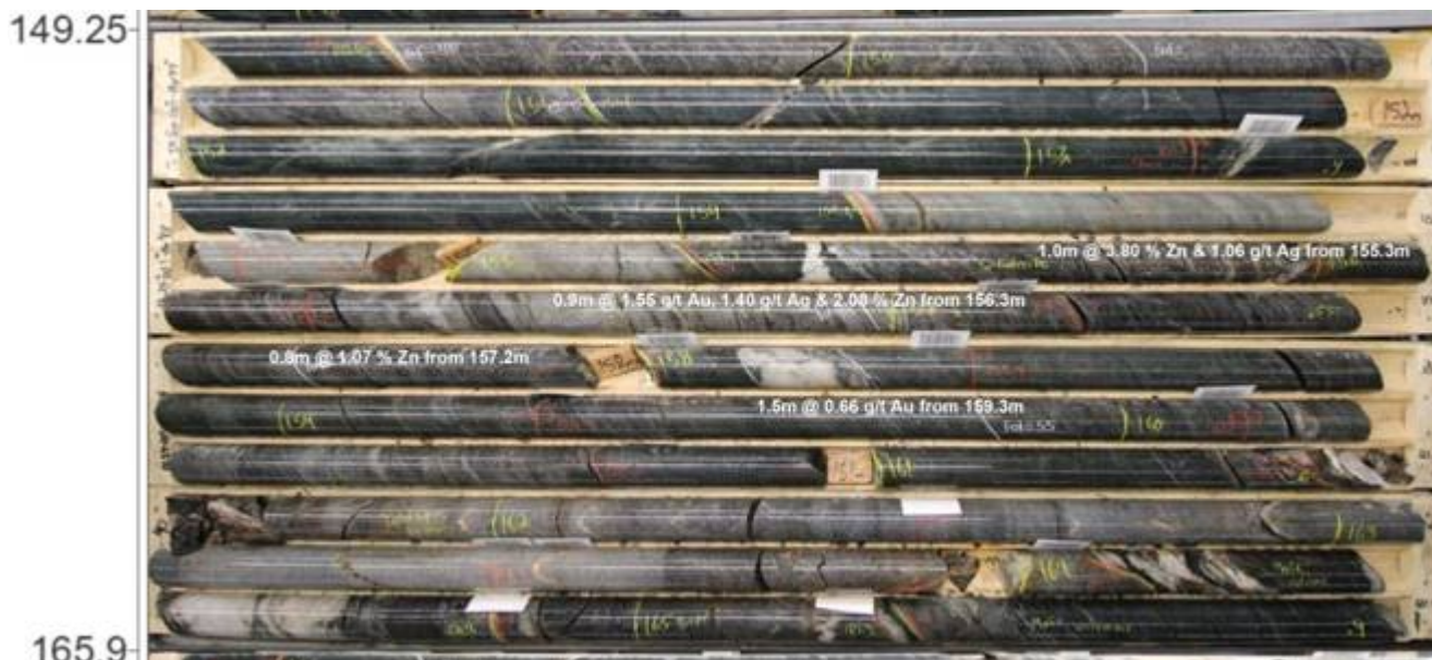
Figure 2: Photography of DL24-001 Drill Core over the interval from 155.3m to 160.8m downhole depth which returned 4.5m @ 0.64g/t Au from 156.3m and 5.5m @ 1.21 % Zn from 155.3m. Photograph markup shows additional high grade intervals such as 1.0m @ 3.80 % Zn & 1.06 g/t Ag from 155.3m, 0.9m @ 1.55 g/t Au, 1.40 g/t Ag & 2.08 % Zn from 156.3m, 0.8m @ 1.07 % Zn from 157.2m and 1.5m @ 0.66 g/t Au from 159.3m.
