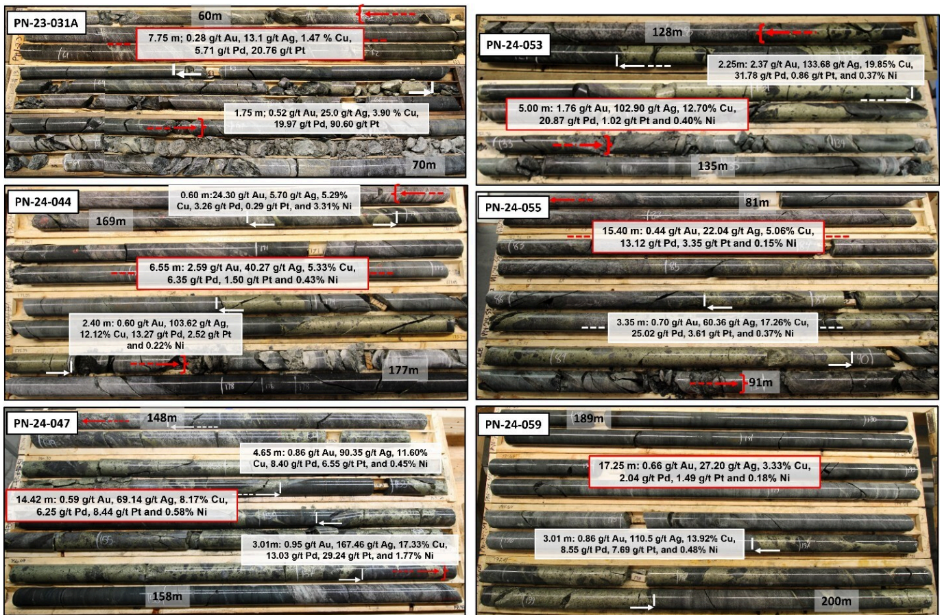
Figure 1: Core pictures showing the relation between observed massive chalcopyrite and grade, and the relative visual amount of massive chalcopyrite (MCp) observed in some the best
