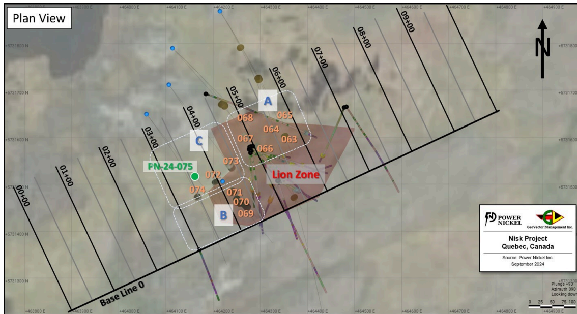
Figure 2: Surface plan view of the Lion Discovery zone; highlighting the location of holes PN-24-063 to PN-24-075. The figure highlights the currently projected size the of the zone. (CNW Group/Power Nickel Inc.)
