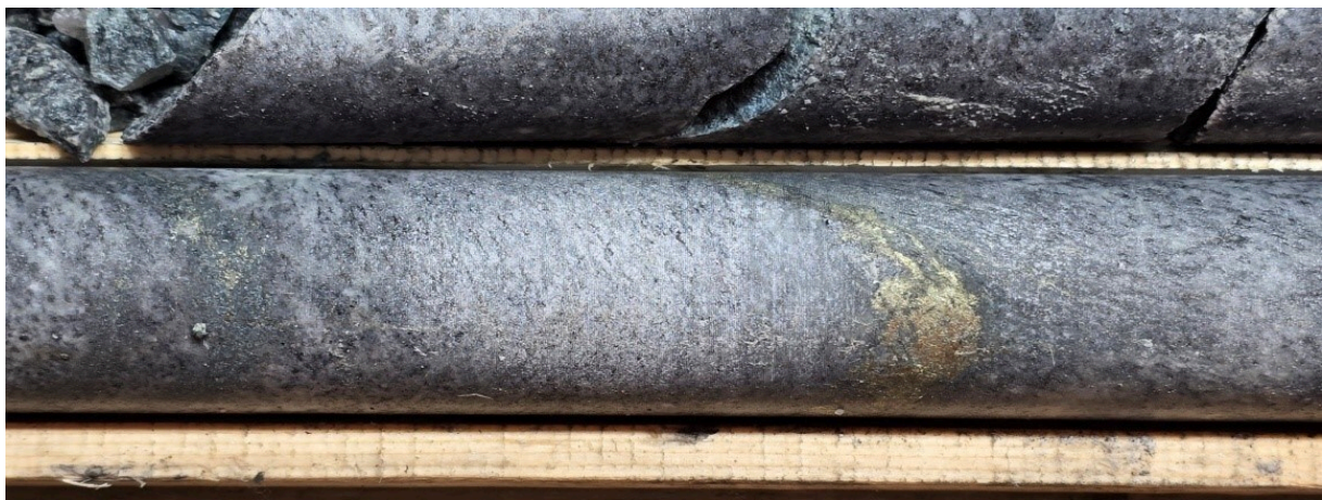
Figure 2: Example of minor Cu mineralization in PN-24-090 drill core that led to BH EM discovery in PN-24-094 (CNW Group/Power Nickel Inc.)
