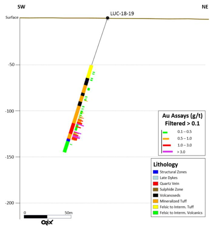
FIGURE 6- LUC 18-19 Drill Hole Section and Graphic Log with Au Assays
