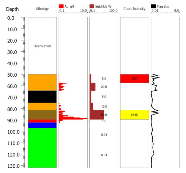
FIGURE 8- LUC 18-21 Drill Hole Section and Graphic Log with Au Assays
