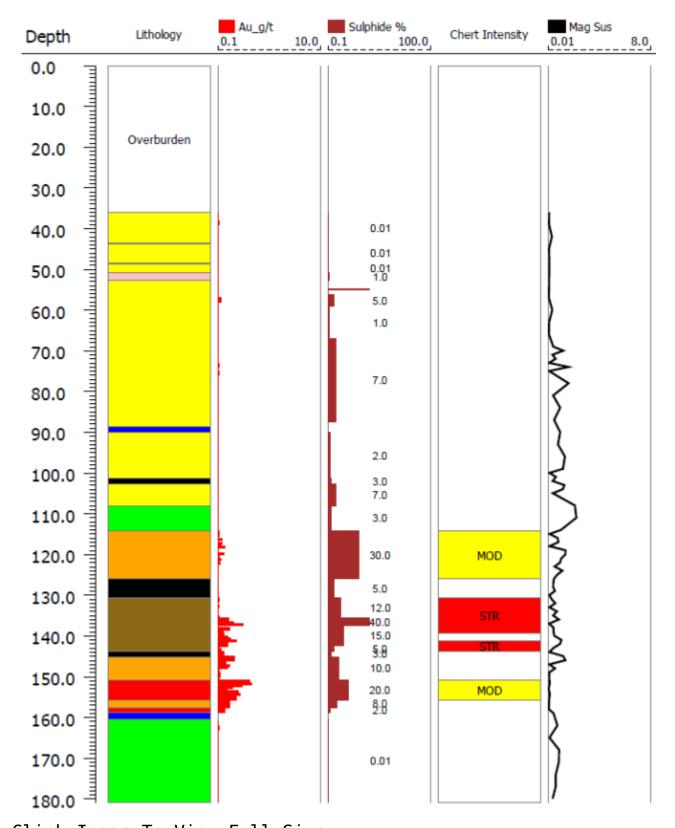
FIGURE 5- LUC 18-14 Drill Hole Section and Graphic Log with Au Assays
