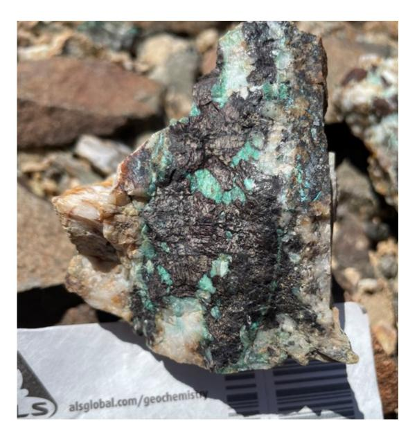
Photo #1 — Sample #E268328 from the "Au-Cu Adits" dump site. Massive, black, tarnished chalcopyrite (copper-iron sulphide) and green secondary copper mineral staining in a white quartz vein. Assayed 1.7 g/t Au. Copper and silver results pending. One of very many such pieces at this site, some assaying up to 17.9 g/t Au.
