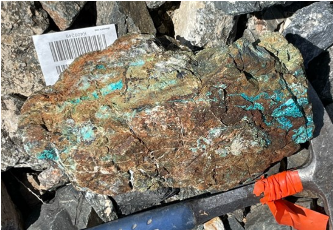
Photo 1: One of the 9 copper-rich boulders sampled on the new claims. Assayed 2.5% Cu, 2.4 g/t Au.
