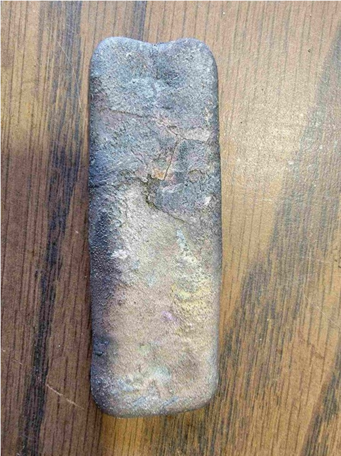
Dore bar poured March 15, 2023.
