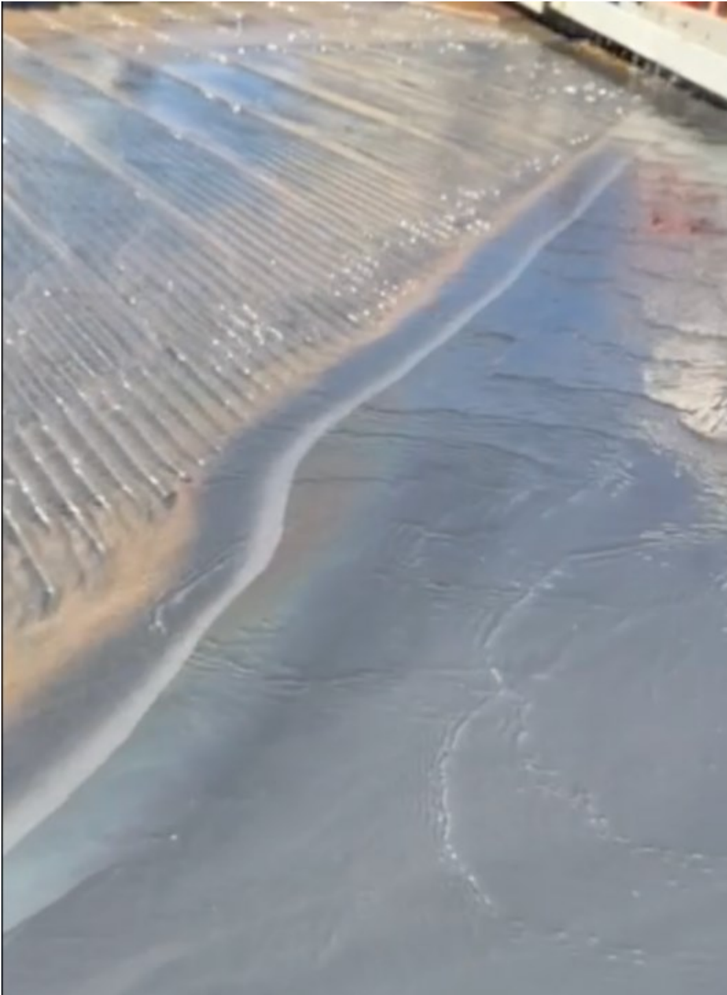
Silver mineralization on shaker table Dec 10, 2023
