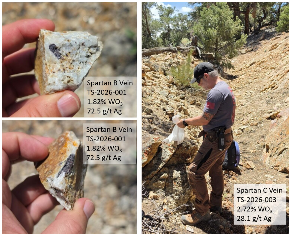
Figure 5 Spartan B and C Vein field samples showing 1-2-centimeter (cm) huebnerite crystals in quartz. Sample bag is sitting on quartz-huebnerite vein at Vein C.
