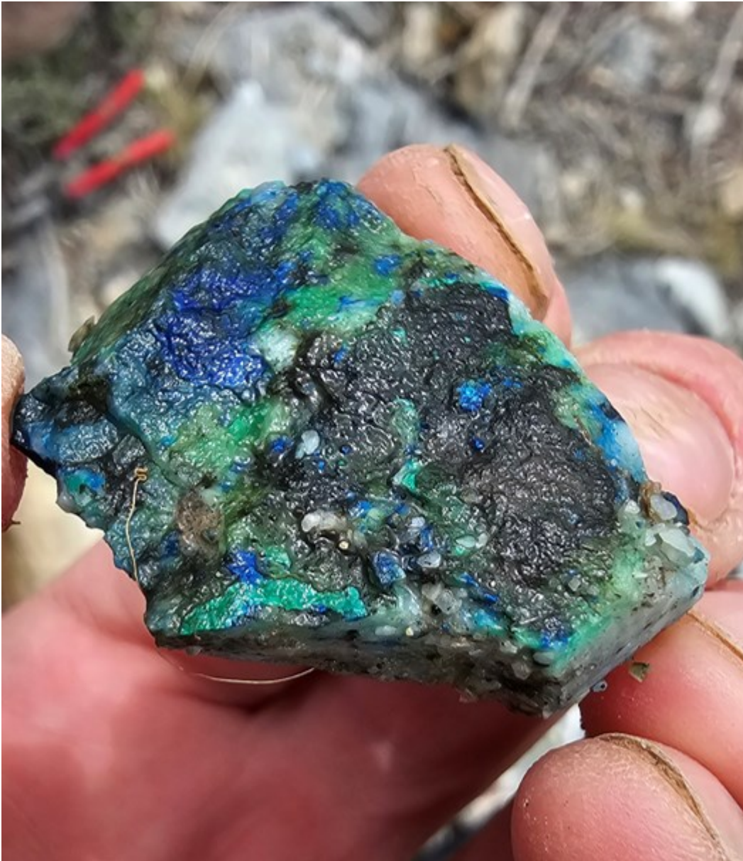
Figure 6 Portion of channel sample (An-2026-001) from near Antelope Mine portal showing malachite (green), azurite (blue), and tetrahedrite (black) minerals that bear the Ag, Cu, and Sb
