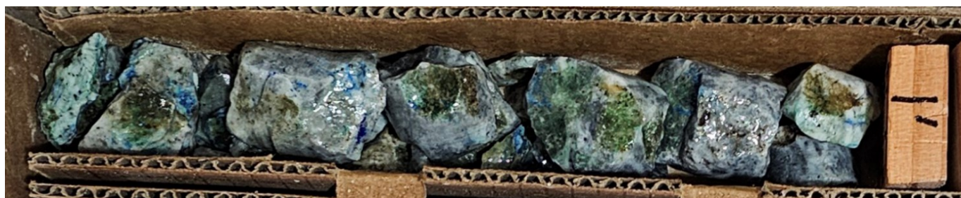
Figure 5 Hole STS-26-008 Antelope vein showing malachite (green), azurite (blue), and tetrahedrite (black specks) minerals that bear the Cu, Ag, and Sb
