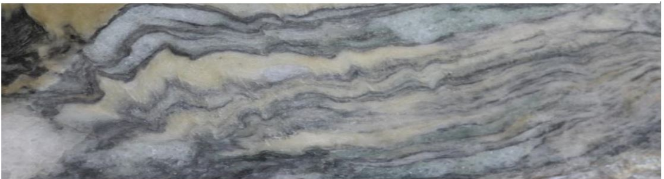
Figure 3 – Grey-White Quartzite produced from test block, VMC Quarry # 4
