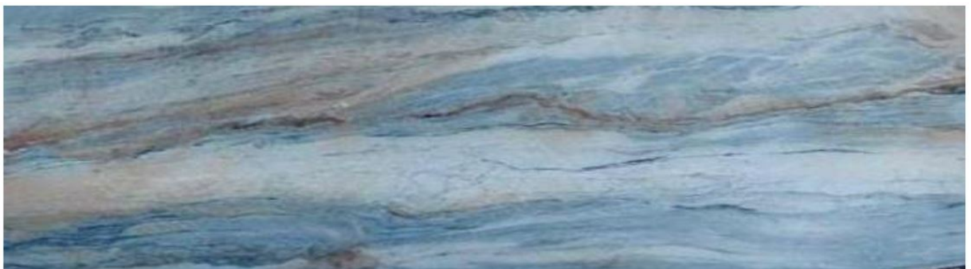
Figure 2 – Blue-Grey Quartzite produced from test block, VMC Quarry # 3
