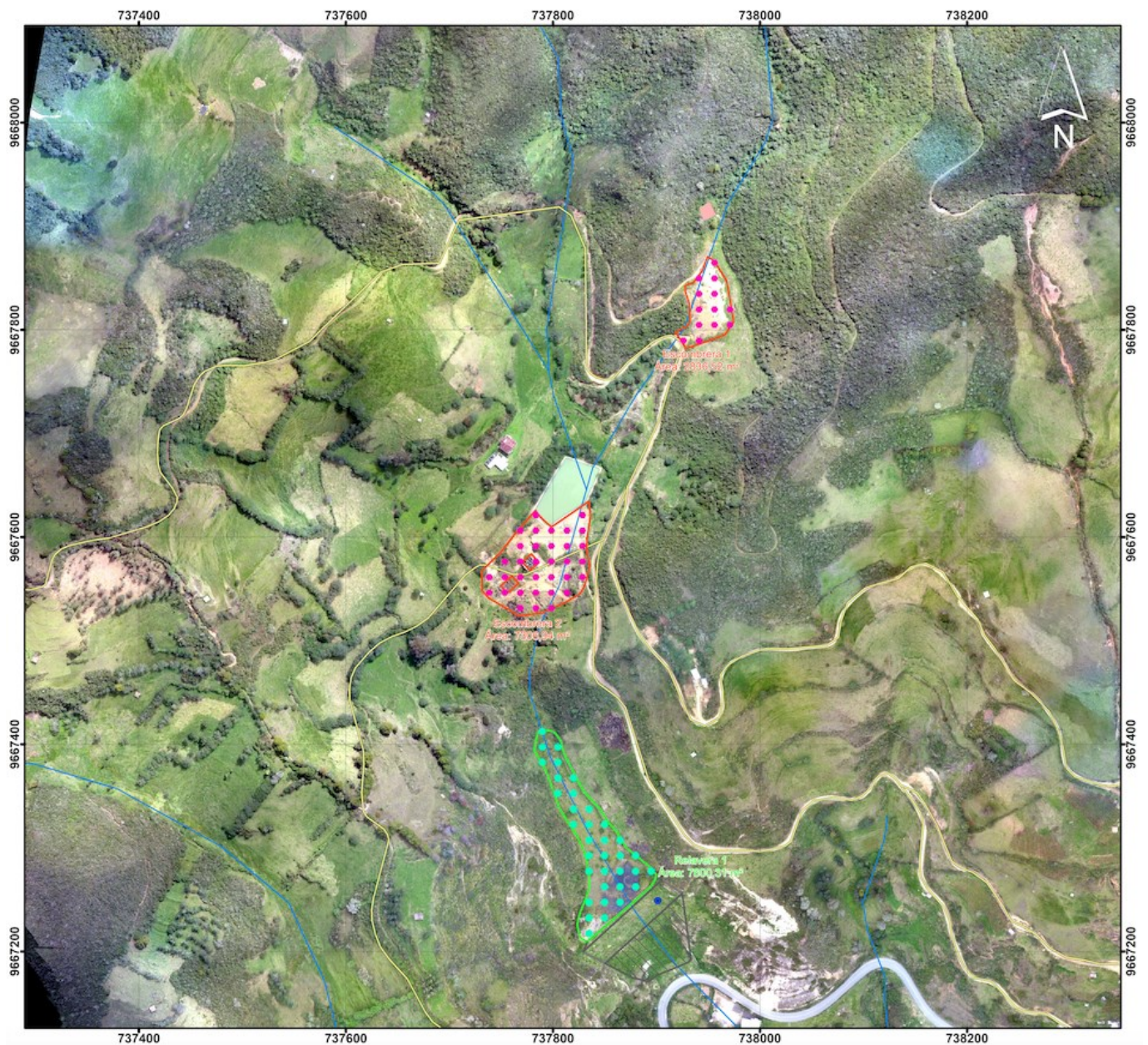
Map of the Silver-1 Mine area showing planned tailings drilling [green] and waste rock sampling [pink]
