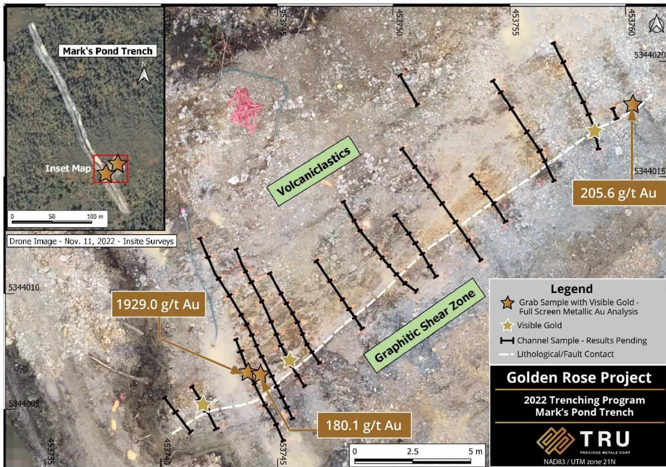
Figure 2: Grab sample results within Mark's Pond trench To view an enhanced version of Figure 2, please visit: https://images.newsfilecorp.com/files/5993/145415_d703970ac4267a6a_002full.jpg
