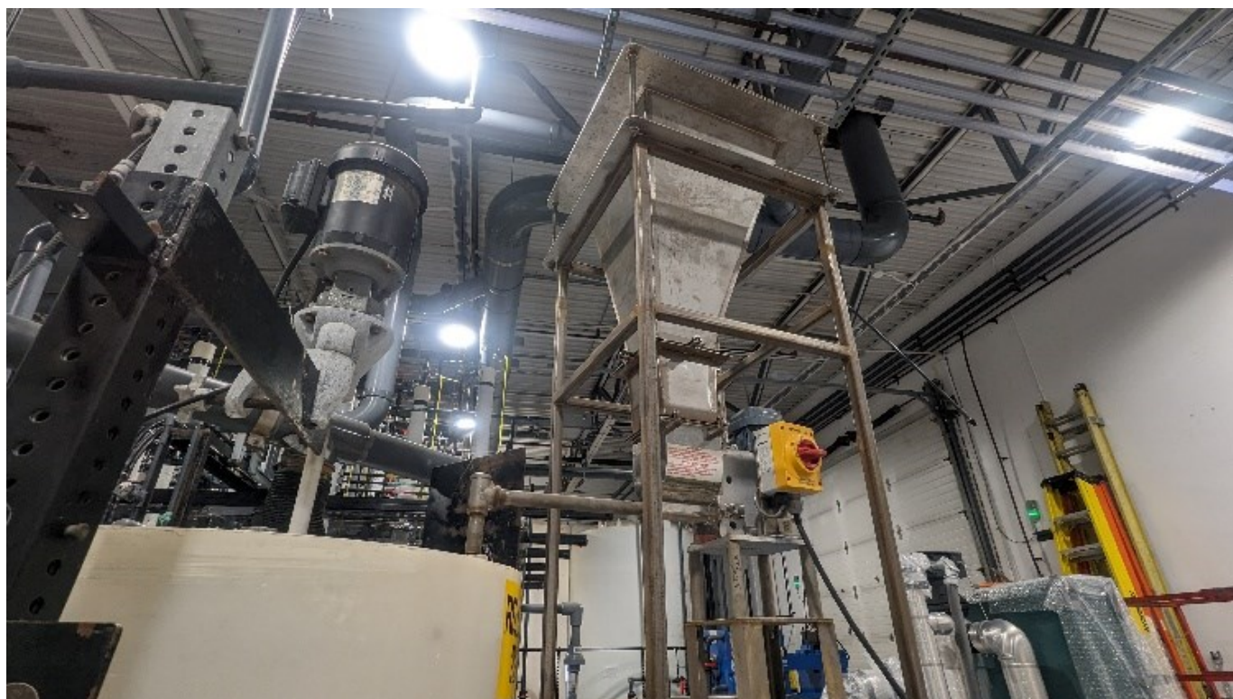
Figure 3 – RapidSX™ Automated Leaching Feeder
