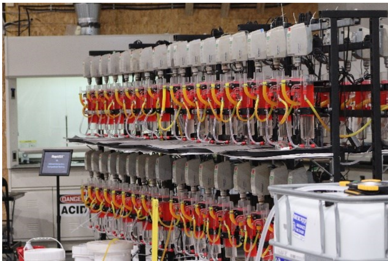
Figure 2 – 52-Stage CSX Pilot Plant
