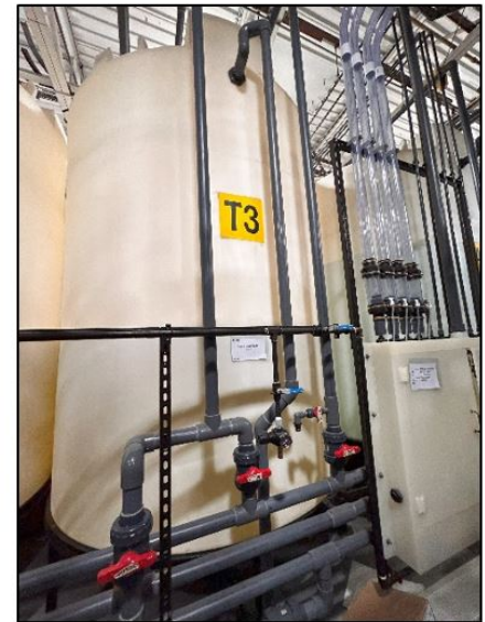
Figure 1: Thousands of liters of separated rare earth chloride products: T5 Raffinate (La, Ce, Pr, Nd, Sm, Eu, Gd, Tb, Dy), T2 Strip One Liquor (Ho, Y, Er, Tm, Yb) and T3 Strip Two Liquor (Yb, Lu) – each tank has a 17,400 liter capacity.
