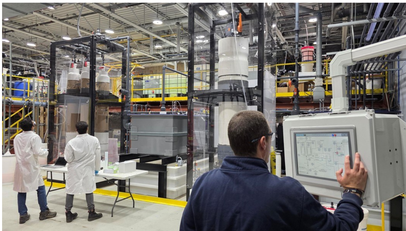
Figure 1: 4×12" (L) & 1×24" (R) RapidSX™ Contactor Scale-Up Testing & Optimization at the Kingston, Ontario, Commercialization and Demonstration Facility
